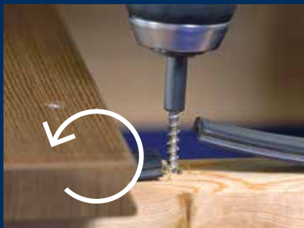
2. Unscrew the remaining part of the screw with the left-bolt extractor in left-hand rotation
