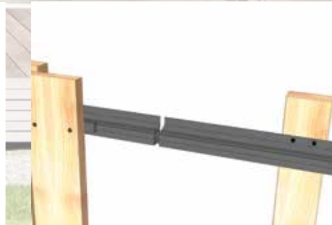
For butt joint of TefaFix® F
