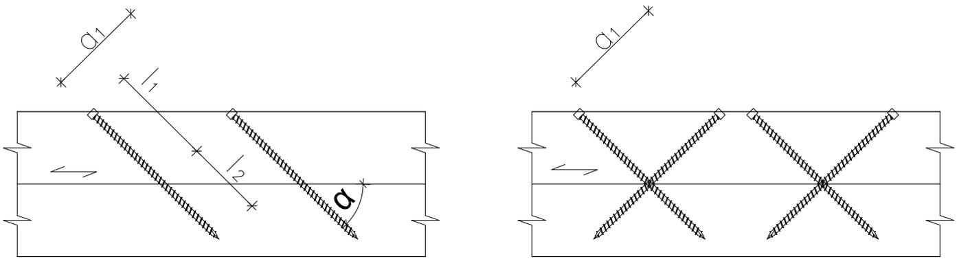
Figure 10: Mechanical jointed beam
