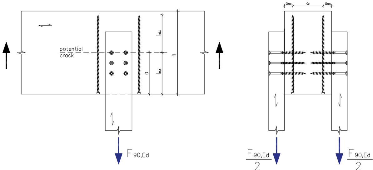
Figure 4: Reinforcement of connection perpendicular to the grain with fully threaded screws
