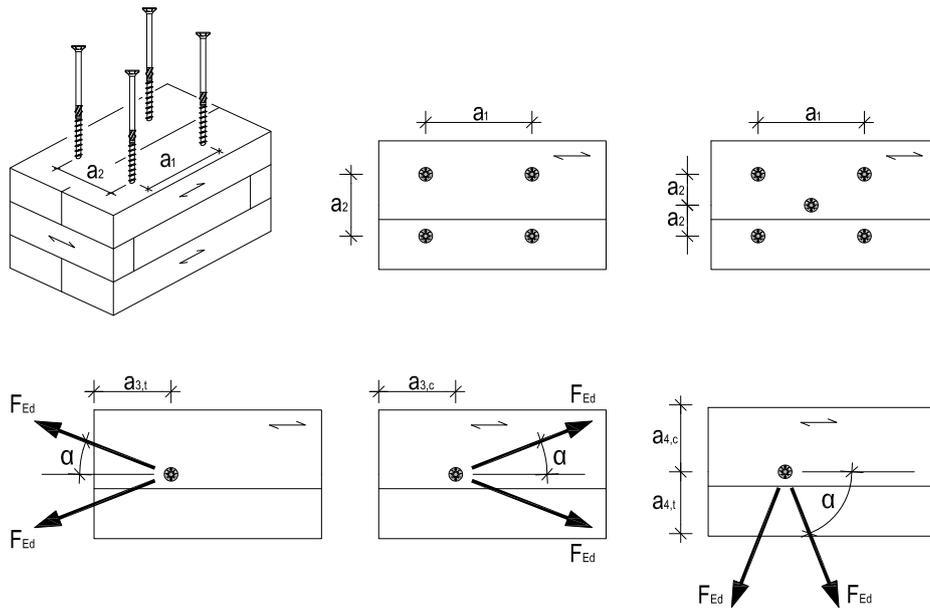
Figure 8: Recommended minimum spacing, end- and edge distances for screws in the plane side of CLT-elements
