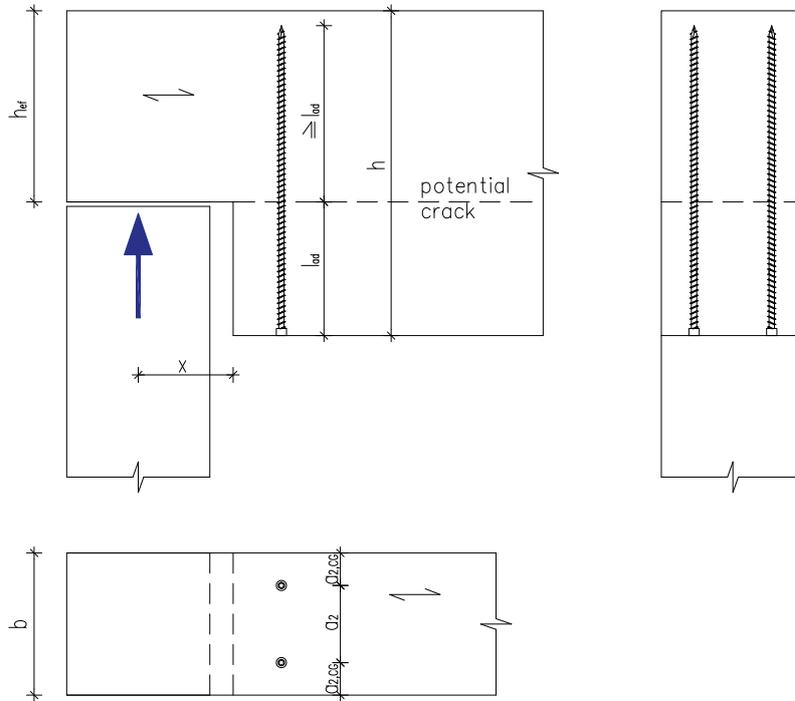
Figure 5: Reinforcement of notched beam support
