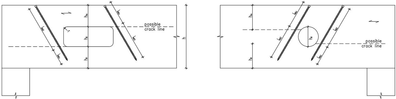
Figure 7: Reinforcement of holes in beams with inclined screws
