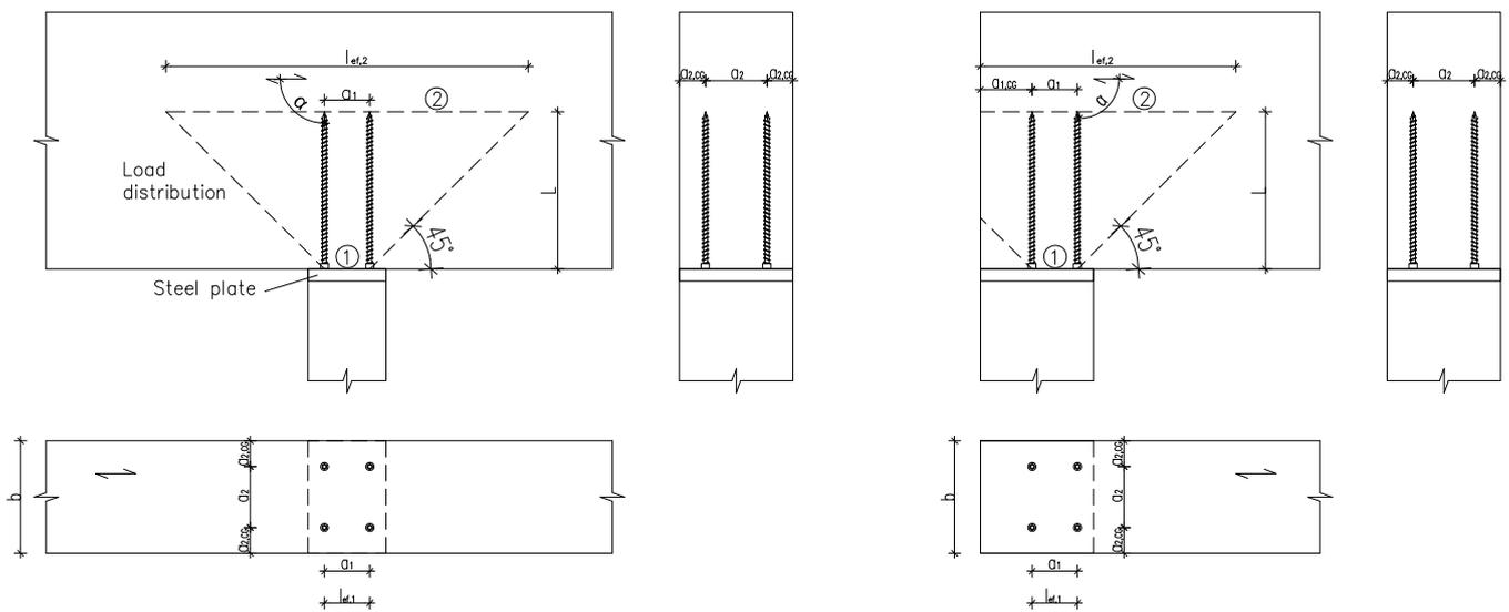
Figure 3: Compression reinforcement perpendicular to the grain with fully threaded screws
