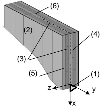
Figure 1: Notations CLT-elements
