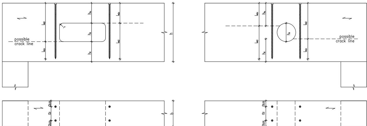
Figure 6: Reinforcement of holes in beams
