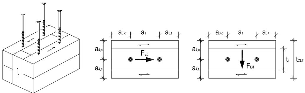
Figure 9: Recommended minimum spacing, end- and edge distances for screws in the narrow side of CLT-elements
