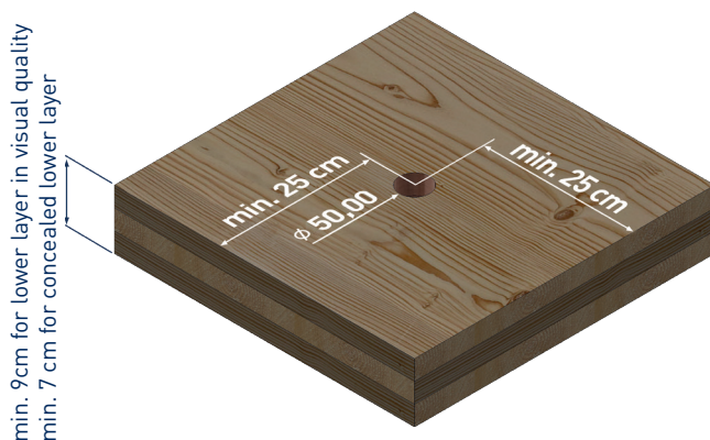
Horizontal manipulation of CLT
