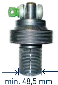
The diameter of the spread element may not be less than 48.5 mm when it is pressed together
