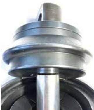
The knee-joint bar must be connected stiff on the top with the hemisphere; the hemisphere and knee-bar joint may not be twisted at all
