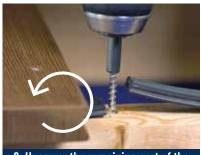
2. Unscrew the remaining part of the screw with the left-bolt extractor in left-hand rotation
