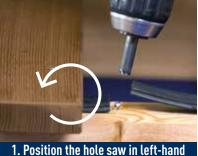
1. Position the hole saw in left-hand rotation and mill off the remainig part of the screw
